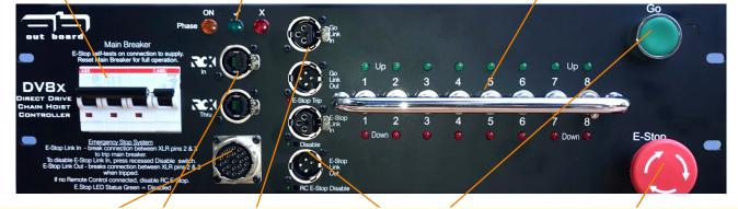
NB: Emergency Stop automatically self-tests by tripping the Main Breaker on connection to supply. Reset Main Breaker to restore operation
