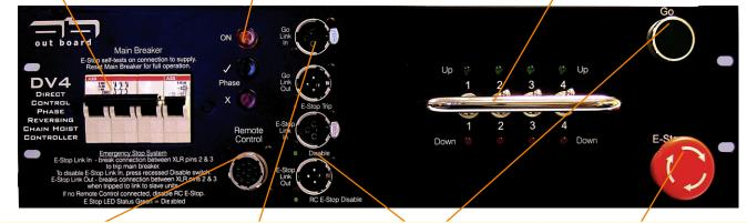
NB: Emergency Stop automatically self-tests by tripping the Main Breaker on connection to supply. Reset Main Breaker to restore operation
