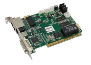
The MSD300, one of the M3 series independent controllers of NovaStar, supports video and audio input. After decoding and data processing, videos and audios can be sent to the screen via Ethernet port. A single controller supports resolutions up to 1920 X 1200@60Hz. It communicates with the computer via USB port, which is convenient to use.
