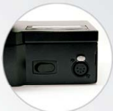
Built-in Wired DMX Control
